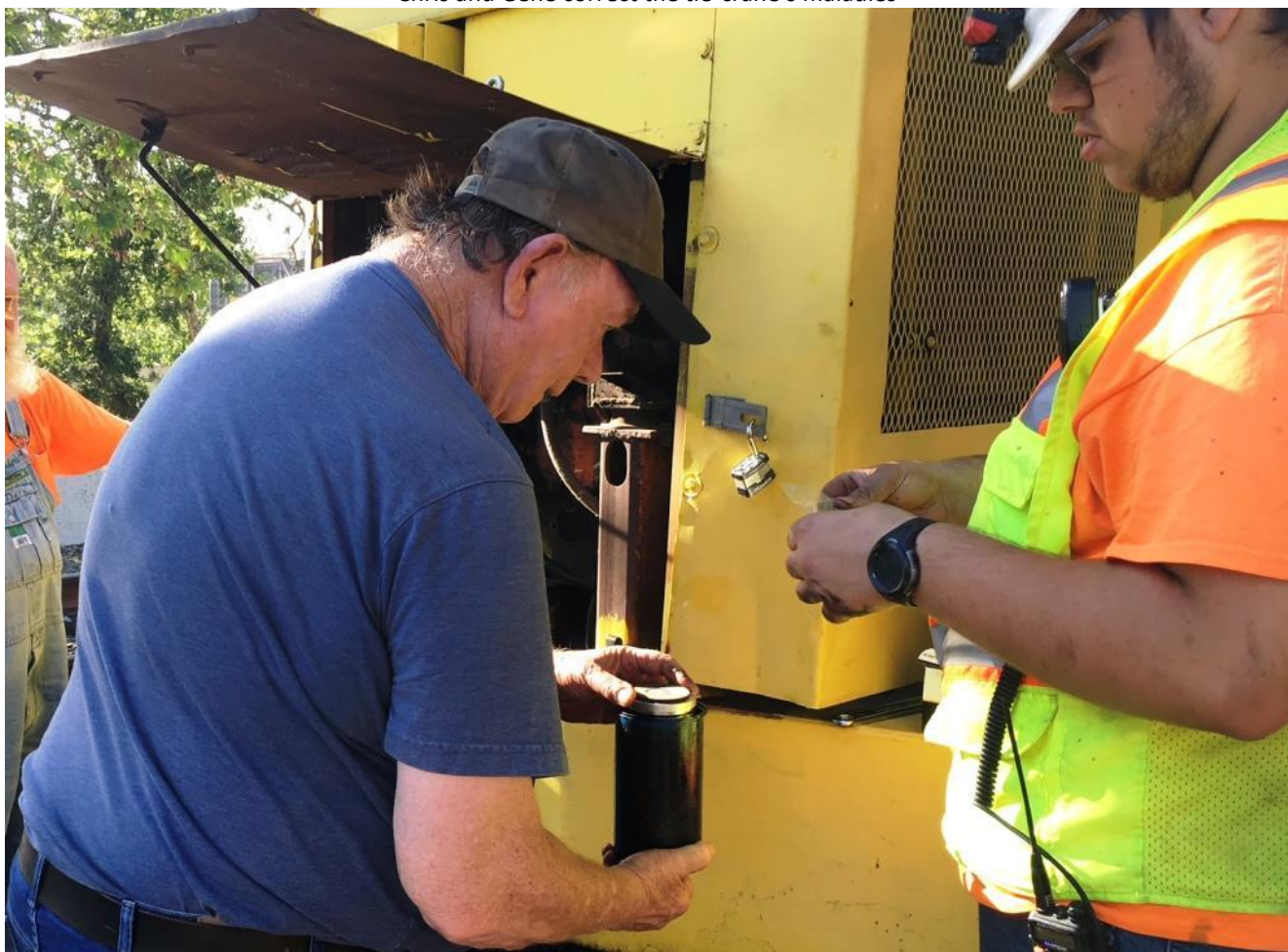
Gene pulls the fuel filter from the tie-crane
